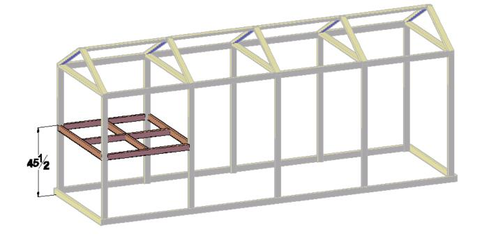
Step 4: Use triplay for the walls. Make a cut out in one wall for the chicken nest 36"x12"
