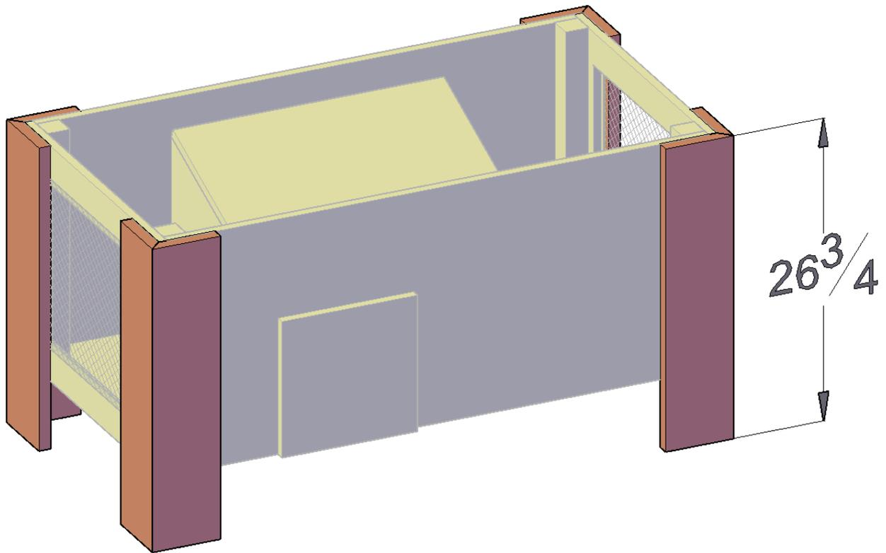
**Step 6:** Use Strap hinges to attach the top roof. Then attach the cover metal roof.
