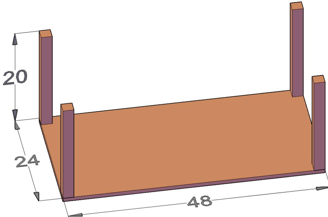
**Step 2:** Attach the Nest boxes together with the following measurements. Use 2x4s as supports.
