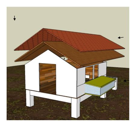
**Step 7:** provide pop door 12"x24" and attach plywood inclined to the ground.
