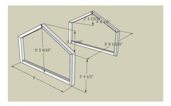
**Step 3:** Prepare Bottom Support as shown in Picture and Attach the wall and frame to the Base.
