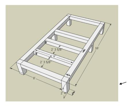
**Step 4:** Use 2x4s to attach the Nest wall and the supports.
