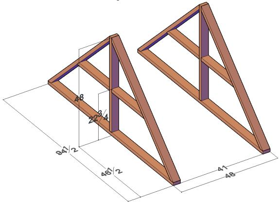
**Step 2:** For supports use 2x4s as shown below and attach with 3" wood screws or nails.
