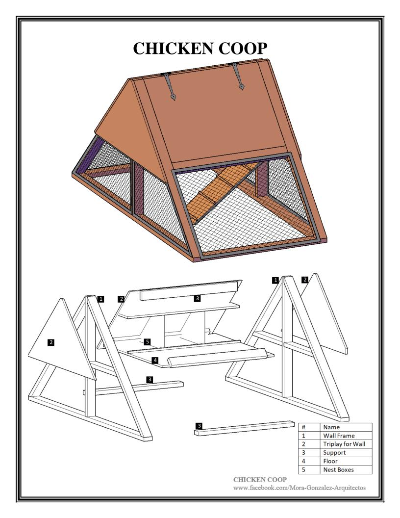
**Step 1:** To build the Frame use 2x4s as shown below, using the 3" wood screws or nails.
