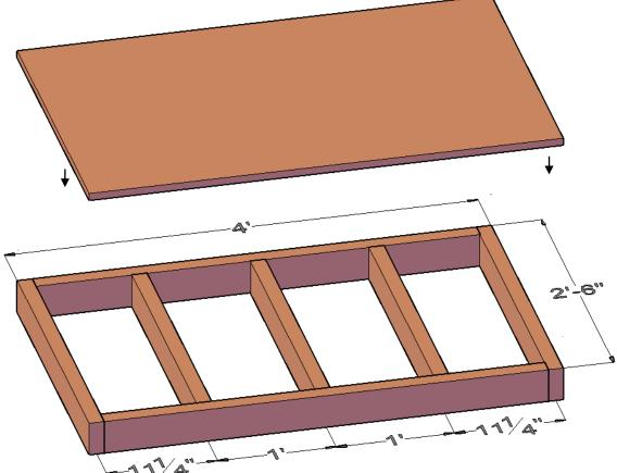
**Step 2:** You will need to frame two side walls. Use 2x2s to build the walls.
