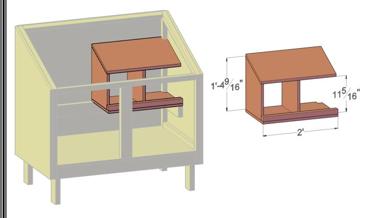
**Step 7:** Cover with triplay the front walls and roof.
