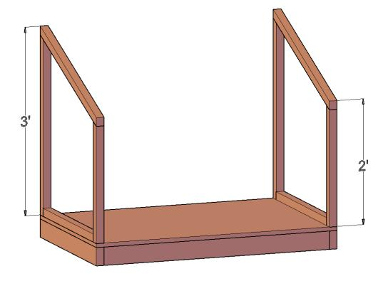
**Step 3:** Use 2x4s and 2x2s to attach the wall supports.
