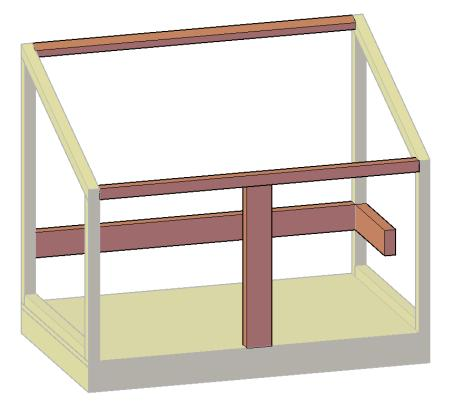
**Step 4:** Use 2x4s for the legs and attach to the floor.
