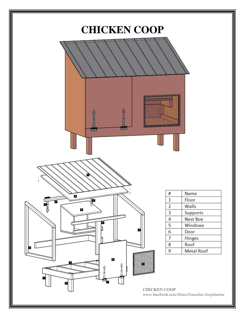
**Step 1:** To build the floor, simply frame up with 2x4s as shown below, using the 3" wood screws or nails.
