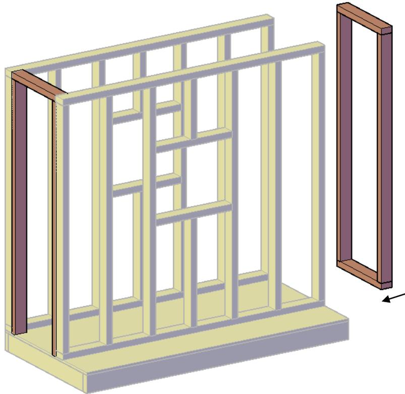
**Step 4:** Use 2x4s to attach the Nest wall and the supports.
