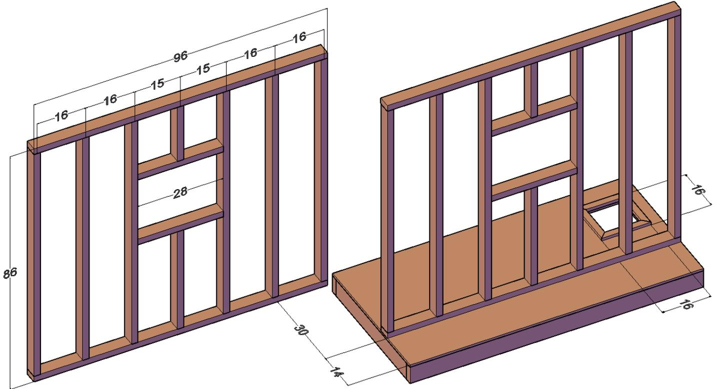
**Step 3:** Use 2x4s to and Attach the wall and frame to the walls.
