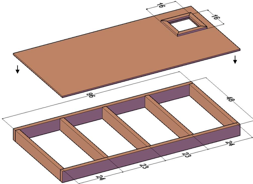
**Step 2:** You will need to frame two side walls. Use 2x4s to build the walls.
